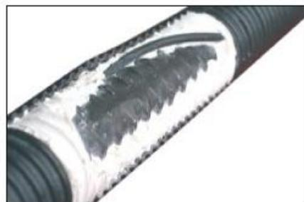
DCP THREADBAR® - exposed section
